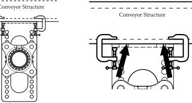
3. Trace the hole locations of the brackets with an indelible ink marker. Remove the full assembly and prepare the surface for drilling.
