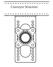
5. Install the brackets and the FGP cleaner together, using FDA-approved 13mm fasteners (not included in the kit). Tighten the fasteners until they seat fully against the metal, then turn 90°.
