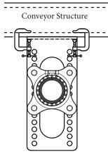
2. Assemble the FGP cleaner to the mounting brackets and clamp it to the conveyor belt structure in the final position where the cleaner will operate.
