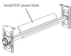
6. Install the plastic blade on the stainless steel pole and verify the belt to blade position. Refer to IOM X3646 to finish the installation.
