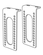
1. Make sure the area where the brackets will be installed is clear of obstructions. The brackets must be installed on a flat surface under the conveyor, preferably on a solid flange.
