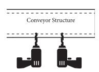
4. Verify that there are no obstructions behind the structure. Back drill two pilot holes first, then enlarge them with a 11/32" (8.5 mm) drill bit.
